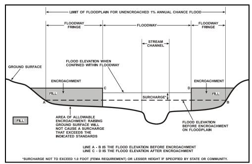
Figure 1 – Floodway Schematic
